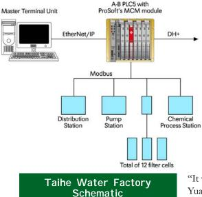
To add the required control, Xu added an Allen-Bradley PLC5/20E with Ethernet capabilities. However, since the original SCADA system was ABB communicating with Modbus, an interface was needed to allow the Modbus end devices to communicate with the Allen-Bradley processor. The solution Xu found was ProSoft Technology's Modbus Communication Module.
